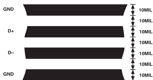
Figure 6. Arrangement of Signal Tracks
